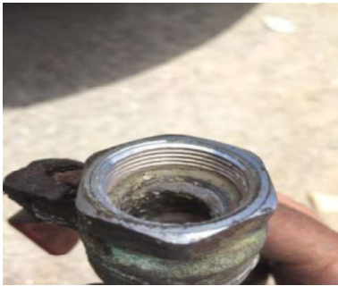
Broken ball valve inside. (Beneteau 26.5)
