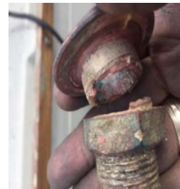
Seacock after being pulled out 3 months later. (Beneteau 26.5)
